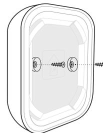
2. Put the siren on the SmartBracket panel and turn it clockwise, then fix the device with a screw.
