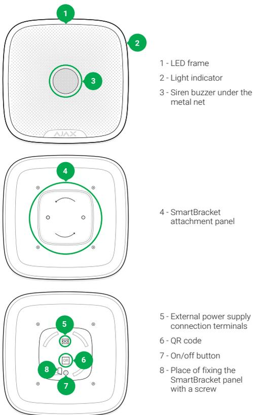
To switch on the siren, press and hold the on/off button for 3 seconds. The siren is switched off in the same manner. If the siren is not linked to the hub, it will automatically power down 6 seconds after activation.
