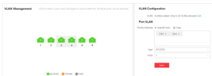
Figure 5-10 Configure Port VLAN
