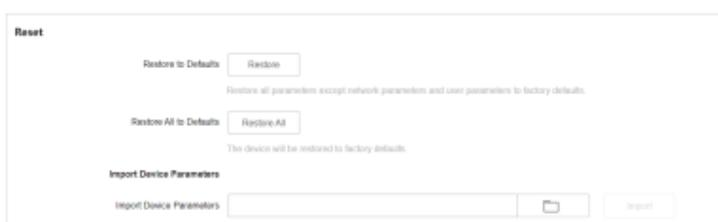
**Figure 6-6 Device Reset**
