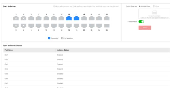
**Figure 5-4 Configure Port Isolation**
