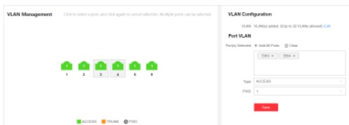
Figure 5-10 Configure Port VLAN
