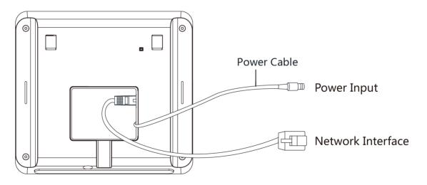
Figure 4-3 Wiring with Power Cable
