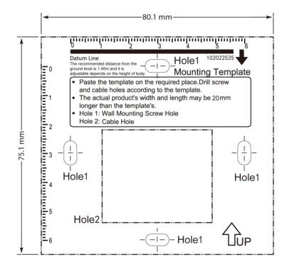
Figure 3-2 Mounting Template
