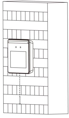
Figure 3-6 Secure Device
