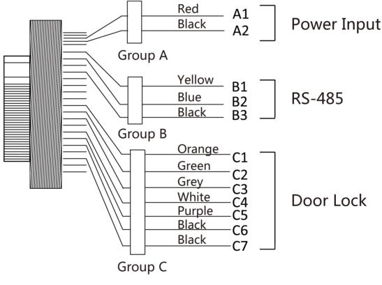
Figure 4-1 Terminal Diagram
