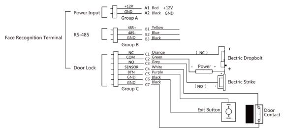
Figure 4-2 Device Wiring
